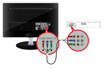
1. Connect the VIDEO OUT port of the AV device (DVD/VCR/Cable/Satellite box) to the [COMPONENT IN [ $P_R$ ,  $P_B$ , Y]] input ports using a component video cable [ $P_R$ ,  $P_B$ , Y].
